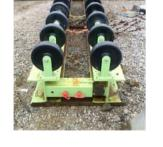
Engineered pipe cutting table jig to stabilize pipe handling and has reduced ergonomic hazards as well
